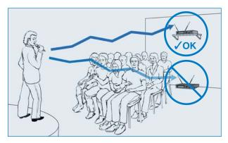
proper and improper antenna and receiver placement
