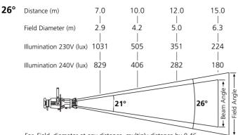
For Field diameter at any distance, multiply distance by 0.46 For Beam diameter at any distance, multiply distance by 0.30
