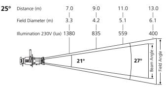
For Field diameter at any distance, multiply distance by 0.44 For Beam diameter at any distance, multiply distance by 0.32
