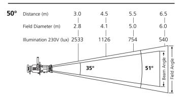
For Field diameter at any distance, multiply distance by 0.89 For Beam diameter at any distance, multiply distance by 0.57
