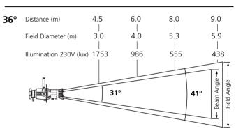
For Field diameter at any distance, multiply distance by 0.67 For Beam diameter at any distance, multiply distance by 0.43
