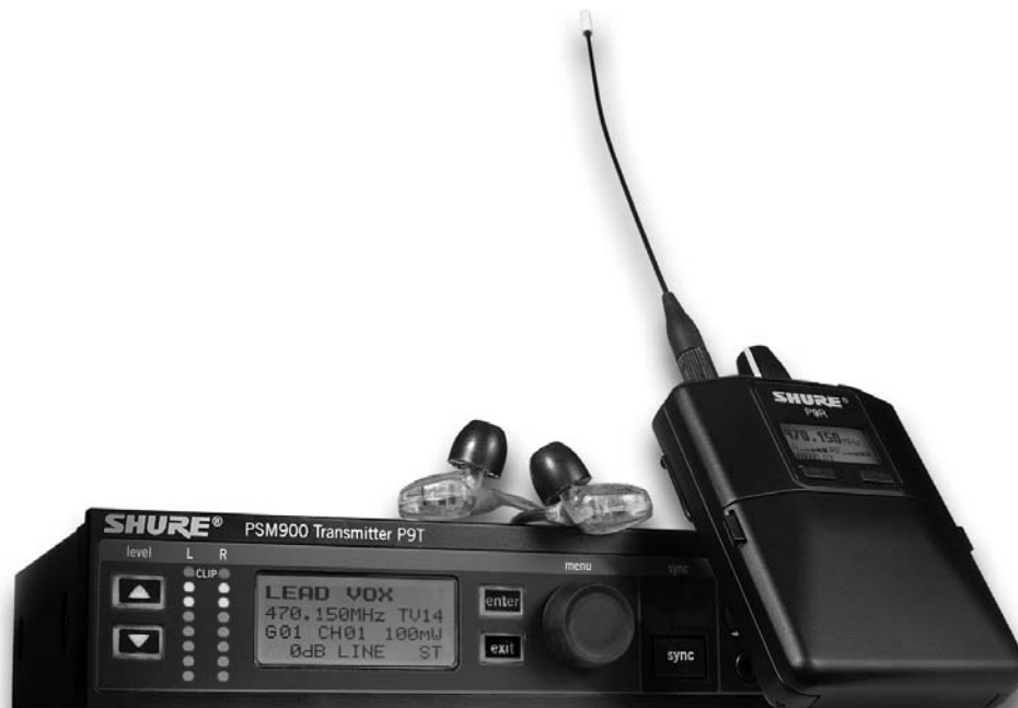
Example of a Personal Stereo Monitor System, including Transmitter, Earphones, and Body-pack Receiver
