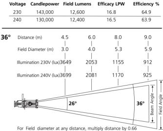
For Beam diameter at any distance, multiply distance by 0.63
