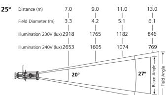
For Field diameter at any distance, multiply distance by 0.47For Beam diameter at any distance, multiply distance by 0.33
