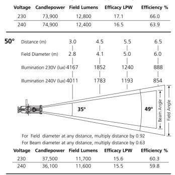
All photometric data in this document was prepared using standard production luminaires, and the Prometric<sup>™</sup> measurement system. Luminaires were adjusted for a flat field and were tested with calibrated HPL 750/230V 19,400 and HPL 750/240V 19,400 lumen lamps at their rated voltage. All data normalised to nominal lamp lumens.
